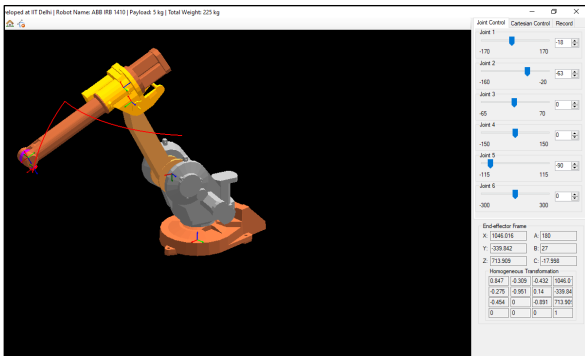
Figure 9. Virtual Robot Module (VRM) of ABB IRB 1410 in RoboAnalyzer.
